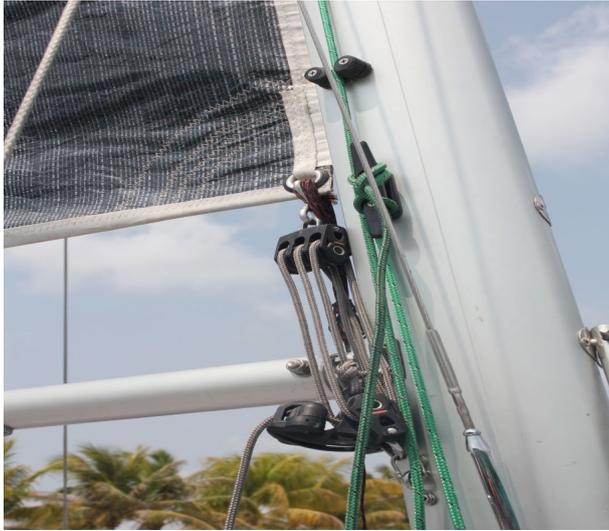
Hoist mainsail to max height by feeding the head of sail into the sail track cut out 150mm on mast just above boom connection. Once you have max hoist lock off halyard using the camcleat and horn cleat on mast, attach the Cunningham hook to the tack and apply a little tension.
