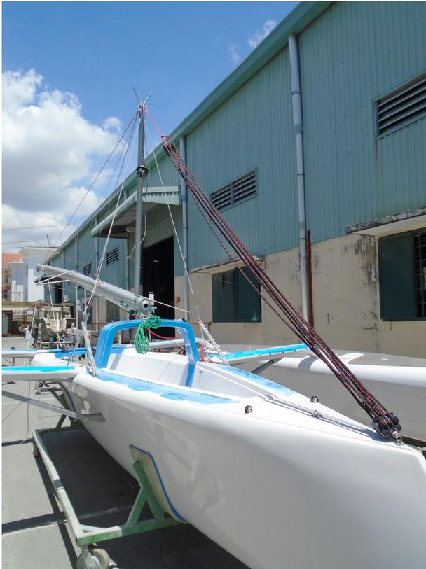
Check to see that all rigging wires are clear and have not snagged anywhere. Raising wires should initially be slightly loose and tighten slightly on the way up.
