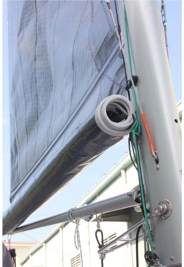
Once you have connected the boom onto mast. Attach the adjustable boom topper onto the rotating SS bracket on the out board end of boom.
