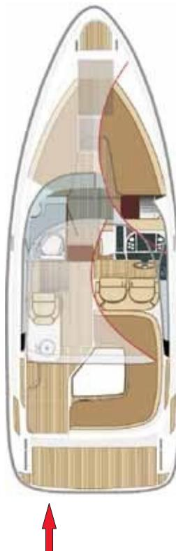
Figure 8. Location of working decks and reboarding ladders.
