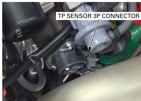
TP SENSOR 3P GRAY CONNECTOR (viewed from the terminal side)
