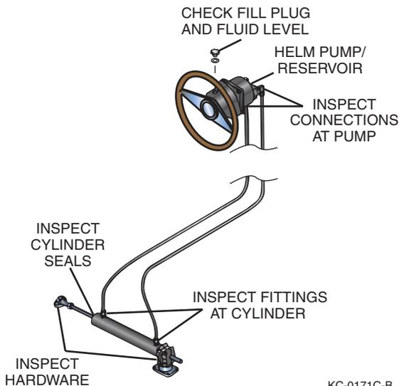
Make sure hydraulic hoses are tight and leak-free. Check cylinder seals for dampness, which indicates leaking. Check the fluid reservoir monthly and top off if necessary. See the steering system manufacturer's information for more details.
