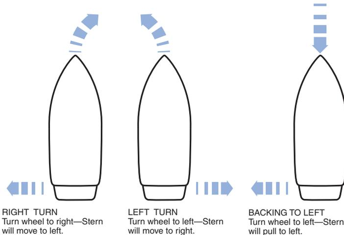
Rotational thrust of the propeller is an aspect most single propeller-driven boats share and needs to be compensated for at slow speeds. During rotational thrust, torque is transmitted to the helm and may cause the boat to drift either port or starboard when moving forward at a slow speed. Rotational thrust usually goes unnoticed at high speeds. While moving forward at a slow speed, constant helm corrections are usually necessary to maintain a straight course.
