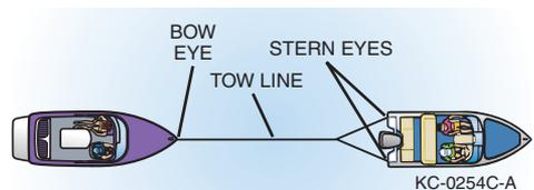
**⚠ WARNING** *Personal Injury Hazard: Use extreme caution when using tow lines and when connecting tow lines to cleats. Death or serious injury could occur if lines and/or cleats fail while they are under extreme tension.*
