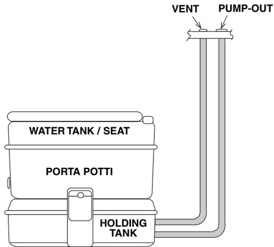
**FIGURE 2.6 – ENCLOSED MARINE HEAD WITH PUMP-OUT**
