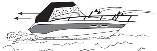
**FIGURE 1.8 DESIRED AIR FLOW THROUGH THE BOAT**
