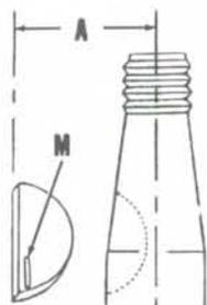
Fig. OM4-7—When installing breaker point cam and flywheel drive key, make certain that the upset mark (M) is down as shown.
