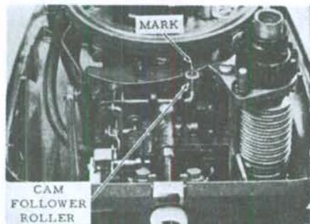
Fig. OM4-2—View of index mark on synchronizer cam aligned with center of cam follower roller.
