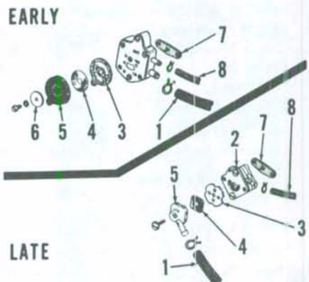
Fig. OM4-5—Fuel pump, fuel filter and associated parts. Early type pump is shown at top.
