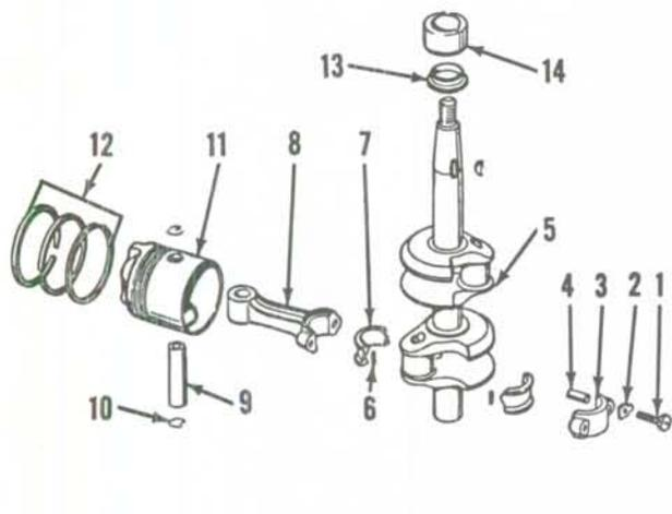
Fig. OM4-13—When attaching connecting rod to crankshaft, make certain that dowels (4) are positioned correctly and 30 bearing needles (6) are in each race. A lip type seal is used in place of slinger (13) on 1967 and late 1966 motors.
