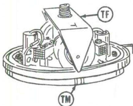
Fig. OM4-6—View of motor with timing fixture (TF) installed. Breaker points should just open when pointer is centered between timing marks (TM) on armature plate.
