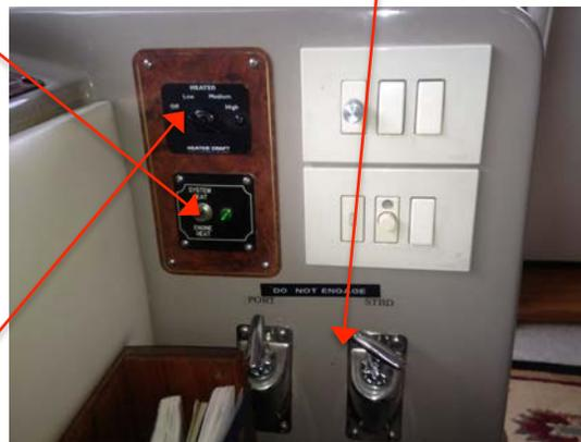
The Pilothouse fan coil unit is located under the bridge and supplies heated air to the window defrosters which can also be operated as just fans using the 3 way manual switch above the Furnace switch
